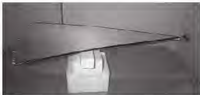
Figure 11.3. A wedge-shaped printed circuit board constructed by Naudin as a test of Dimitriou's experiment. (Courtesy of J.-L. Naudin, from his website. http://jlnaudin.free.fr/ )
