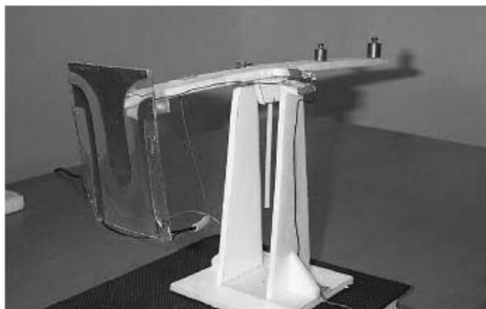
Figure 12.15. A test of the Lafforgue thruster carried out by Jean-Louis Naudin. (Photo courtesy of J.-L. Naudin, from his website, http://jnaudin.free.fr/ )
